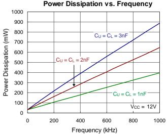
Figure 4. Power Dissipation vs. Frequency
