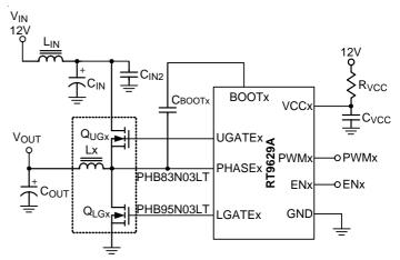
Figure 6. Synchronous Buck Converter Circuit
