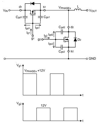
Figure 1. Equivalent Circuit and Waveforms ( $V_{CC} = 12V$ )
