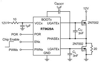
Figure 3. Power Dissipation Test Circuit
