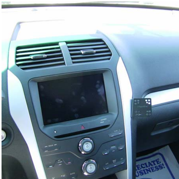
InDash installed showing location
