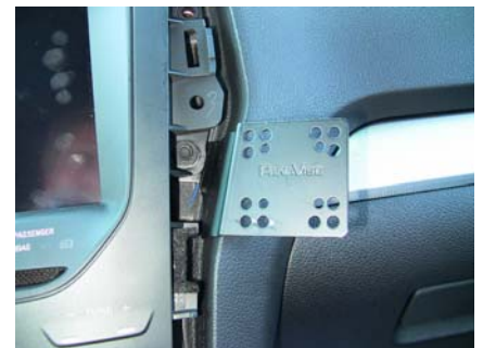
Mount installed showing screw location
