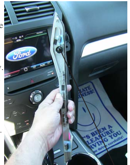
Bezel removal (plastic lug)
