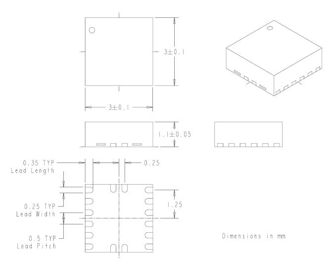
Figure 8. EP5388QI Package Dimensions.
