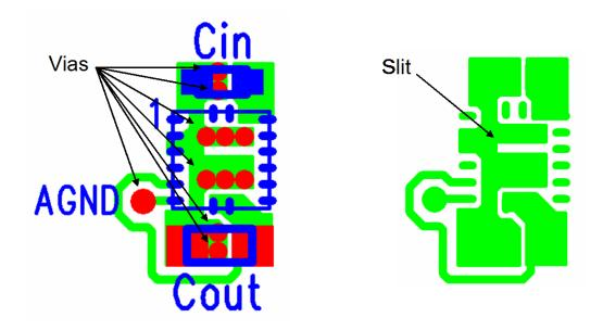
Figure 6. PCB layout recommendation.
