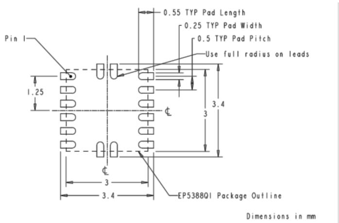
Figure 7. Recommended PCB Footprint.
