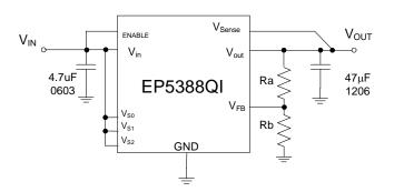
Figure 4. External Divider application circuit.
