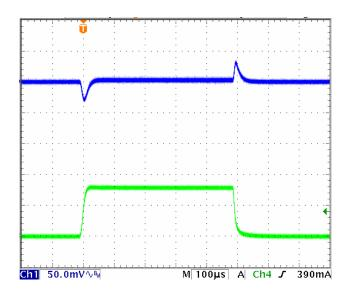
**Transient,**  $V_{IN} = 3.3V$ ,  $V_{OUT} = 1.8V$ , Load = 0-800mA.
