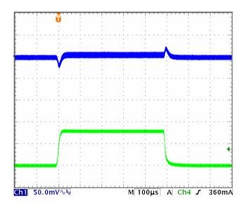
**Transient,**  $V_{IN} = 5.0V$ ,  $V_{OUT} = 3.3V$ , Load = 0-800mA.
