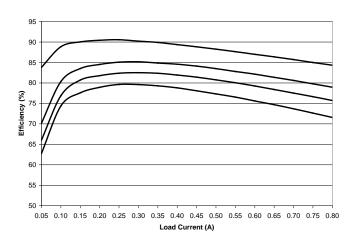
**Efficiency**,  $V_{IN} = 3.3V$ ,  $V_{OUT} = 1.2V$ , 1.5V, 1.8V, 2.5V.
