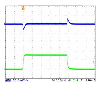
**Transient,**  $V_{IN}$  =3.3V,  $V_{OUT}$  = 1.2V, Load = 0-800mA.
