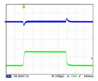
**Transient,**  $V_{IN} = 5.0V$ ,  $V_{OUT} = 1.2V$ , Load = 0-800mA.
