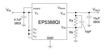
**Figure 5.** Applications circuit for  $C_{OUT} = 1 \times 10 \text{uF} 0805$ .
