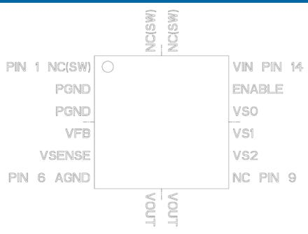
Figure 2. EP5388QI Package Pin-out.
