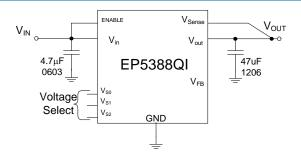
Figure 1. Typical application circuit.
