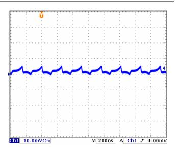
**Output Ripple**,  $V_{IN} = 5V$ ,  $V_{OUT} = 2.5V$ ; Load = 500mA.
