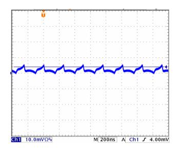
**Output Ripple**,  $V_{IN} = 5V$ ,  $V_{OUT} = 1.8V$ ; Load = 500mA.
