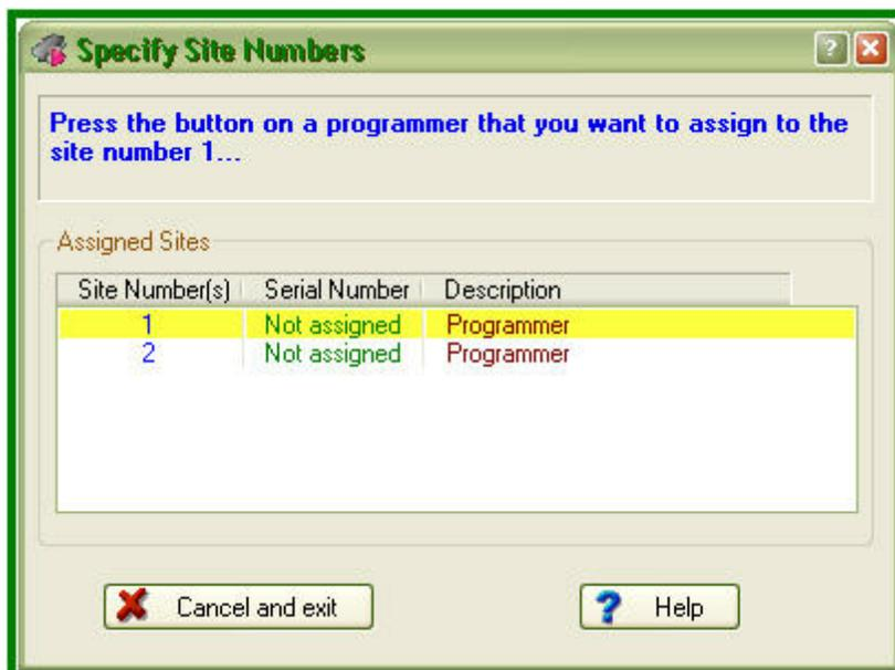
Now you should press the button on the programmer to which you would like to assign the site #1. Then the ChipProgUSB will prompt to assign the site #2 to another programmer (in case there are more than two programmers in the programming cluster), etc. After assigning numbers to the programmers you will get the [Program Manager](#) window that differs from the same window that you get when you work with one programmer.
