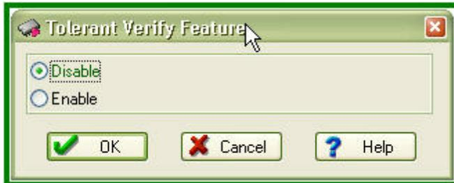
Usually this option is applicable in case of use the [Error Checking and Correction](#) (ECC) method of managing invalid blocks when you can tolerate with some errors in the data fetched from the memory device. When you select **Enable** in the dialog above [Acceptable number of errors](#) dialog:
