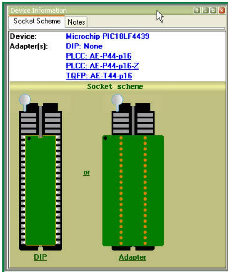
The adapter part numbers are linkable and the links being clicked opens the [adapters.chm](#) file with a description and wiring diagram of the chosen adapter. The cable adapters for in-system programming are also included into the [adapters.chm](#) file. There are some peculiarities that such ISP adapters use depending on the target device type.
