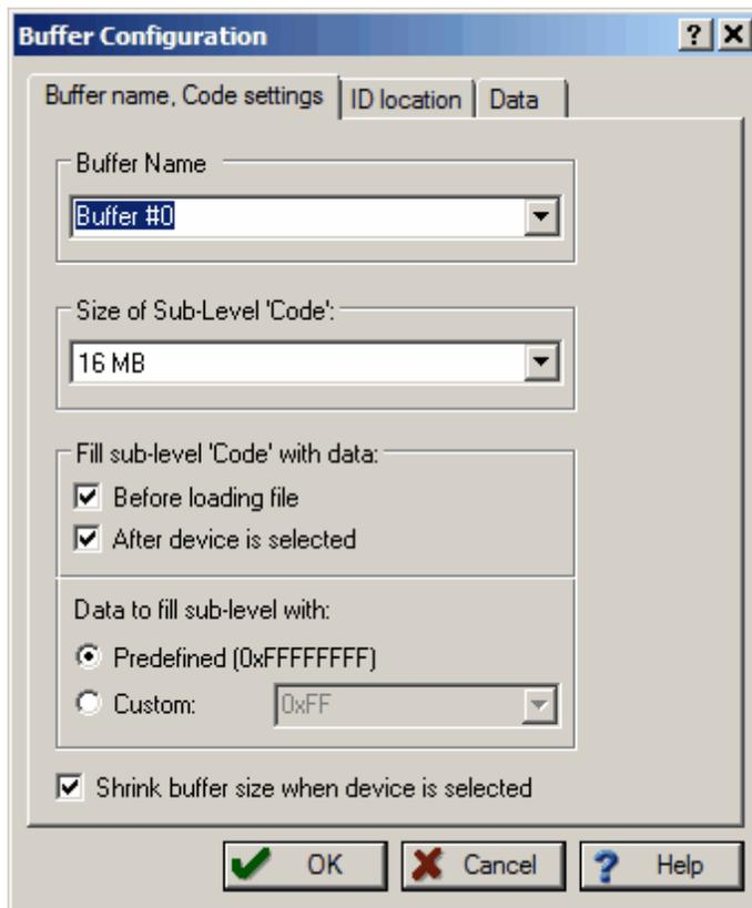
By default each buffer has a minimal size of 128K RAM in a PC and by default the program fills the buffer with a predefined value (usually 0FFh). You can customize these buffer settings - check the Custom radio button and type in the pattern to fill the buffer.
