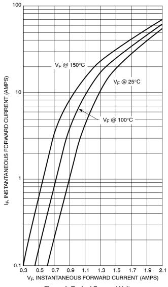
Figure 2. Typical Forward Voltage
