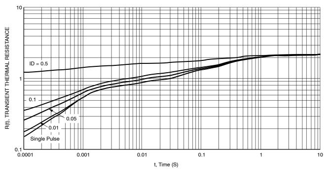
Figure 14. Transient Thermal Response
