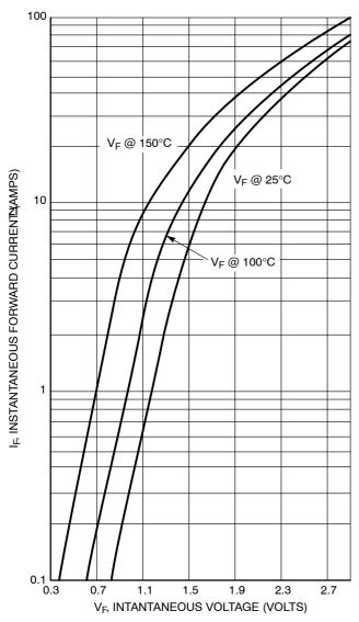
Figure 1. Maximum Forward Voltage
