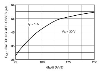
Figure 13. Typical Switching Off Losses
