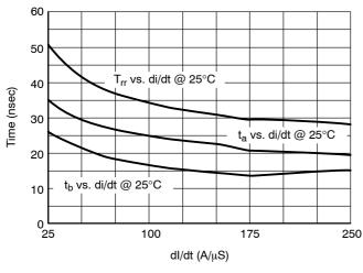
Figure 9. Typical Trr vs. di/dt
