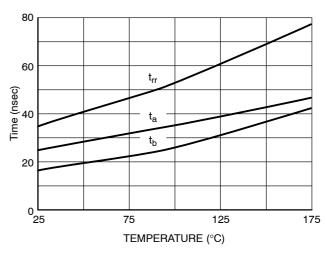
Figure 10. Typical Trr vs. Temperature
