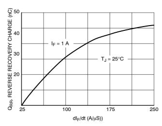
Figure 12. Typical Reverse Recovery Charge
