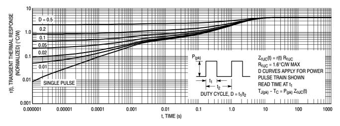
Figure 15. Thermal Response, (MSRF1560) Junction-to-Case ( $R_{\theta JC}$ )
