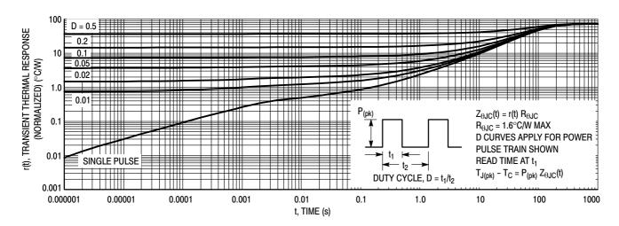
Figure 16. Thermal Response, (MSRF1560) Junction-to-Ambient ( $R_{\theta JA}$ )
