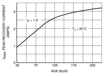
Figure 11. Typical Peak Reverse Recovery Current
