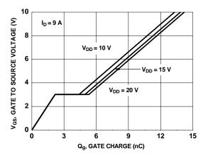
Figure 7. Gate Charge Characteristics
