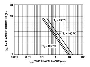
Figure 9. Unclamped Inductive Switching Capability
