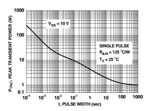
Figure 12. Single Pulse Maximum Power Dissipation
