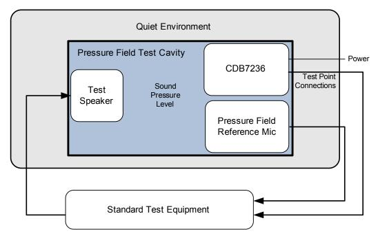
Figure 2-1. Pressure field test setup with CDB7236
