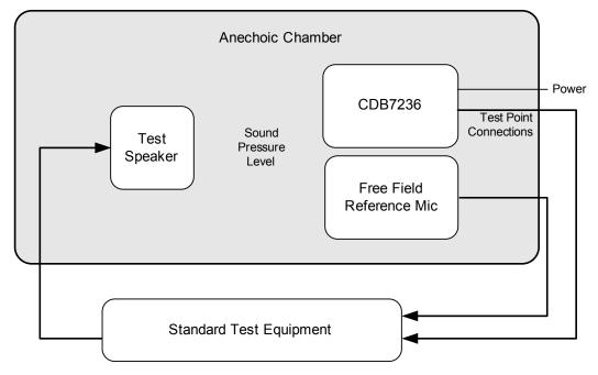
Figure 2-2. Free field test setup with CDB7236
