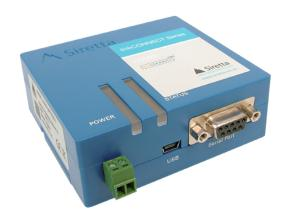
Figure 7. LC200 power, USB & RS232 interfaces
