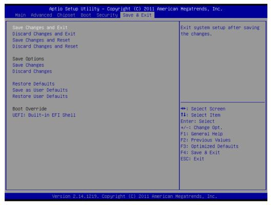
Figure 3.15 Save & Exit configuration setup screen
