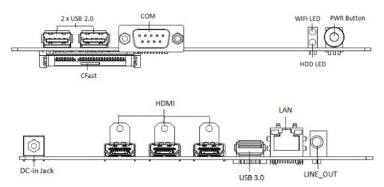
Figure 2.1 Front and rear view
