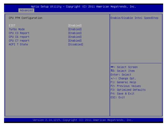
Figure 3.12 CPU PPM Configuration setup screen
