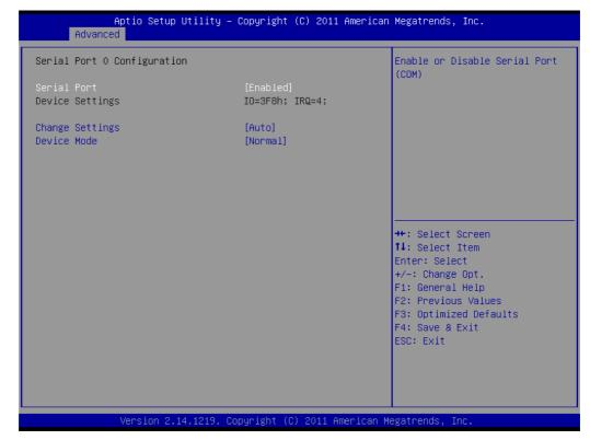
Figure 3.10 Serial Port 0 Configuration setup screen
