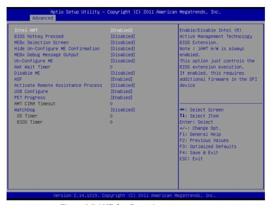
Figure 3.7 AMT Configuration setup screen
