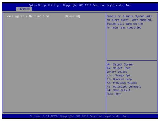
Figure 3.3 S5 RTC Setup Screen
