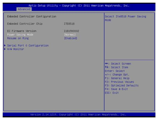
Figure 3.9 Embedded Controller Configuration setup screen
