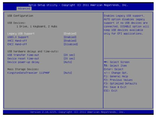
Figure 3.8 USB Configuration setup screen
