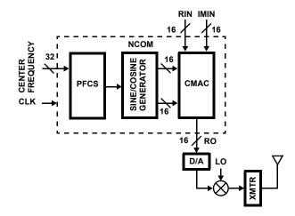
FIGURE 5. QUADRATURE AMPLITUDE MODULATION (QAM)
