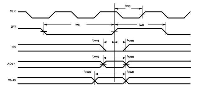
FIGURE 8. CONTROL BUS TIMING
