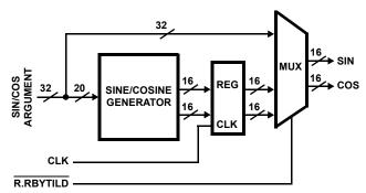
FIGURE 2. SINE/COSINE SECTION
