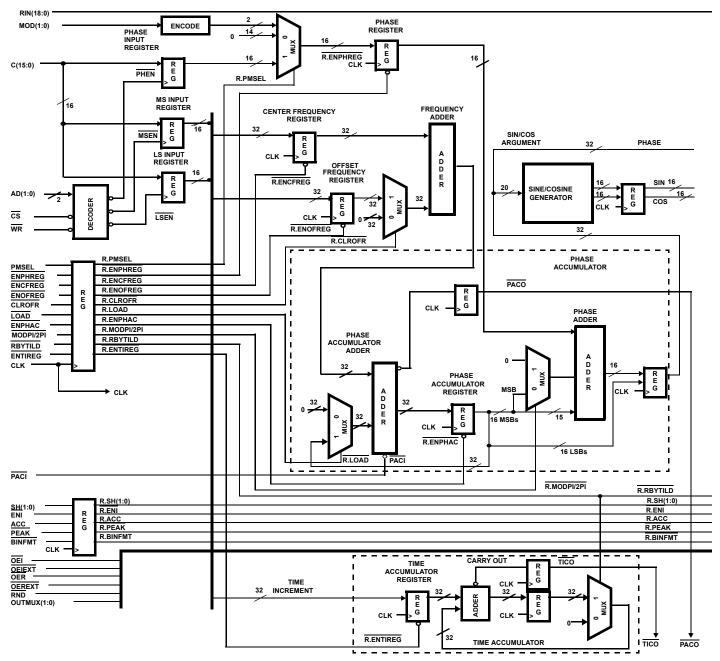
FIGURE 1. HSP45116A BLOCK DIAGRAM
