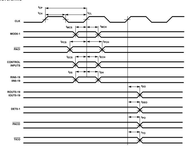
FIGURE 7. INPUT AND OUTPUT TIMING
