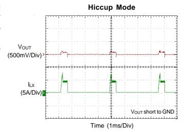
Figure 5. Hiccup Mode Under Voltage Protection
