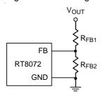
Figure 1. Setting the Output Voltage
