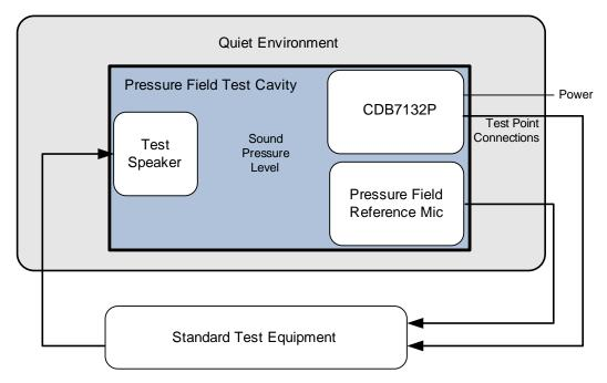
Figure 2-1. Pressure field test setup with CDB7132P
