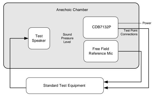
Figure 2-2. Free field test setup with CDB7132P
