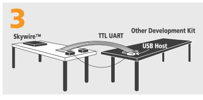
To connect the kit to a different processor or development kit, a 14-pin header breaks out the necessary signals for easy connection to any device. The modem supports I/O levels from 1.65-5.5V, simplifying connection to other systems.
