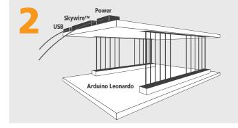
The baseboard is an Arduino shield, so you can plug the module directly onto an Arduino microcontroller. (Kit includes sample sketches showing how to initialize the modem, make data connections, and send and receive SMS messages.)
