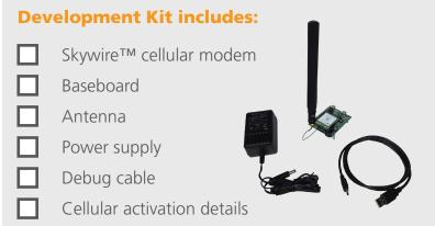
The kit enables you to develop your application directly on the Skywire™ modem with three different ways to connect:
