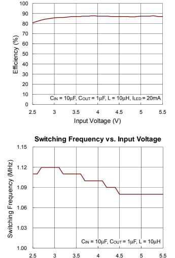
Efficiency vs. Input Voltage
