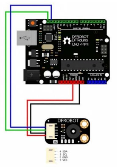
IR Thermometer Sensor-MLX90614 Wire Diagram
