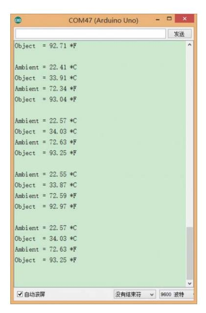
IR Thermometer Sensor-MLX90614 Test Result
