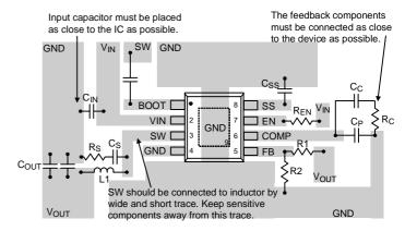
Figure 8. PCB Layout Guide
