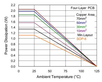
Figure 7. Derating Curves for RT8294 Package
