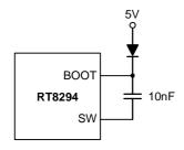
Figure 2. External Bootstrap Diode
