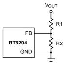
Figure 1. Output Voltage Setting
