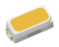
LUXEON 3014 is an industry standard compatible footprint for ease of installation into existing 3014 sockets and stays consistent with a 3.0mm x 1.4mm x 0.75mm package. LUXEON 3014 is hot-color targeted at operating conditions—65°C. This low power device is an ideal choice when uniformity and reduction in spottiness is necessary for indoor designs.
