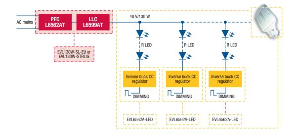
The PFC stage, working in transition mode, acts as pre-regulator and powers the resonant stage with an output voltage of 450 V. The PFC power topology is a conventional boost converter, connected to the output of the rectifier bridge.
