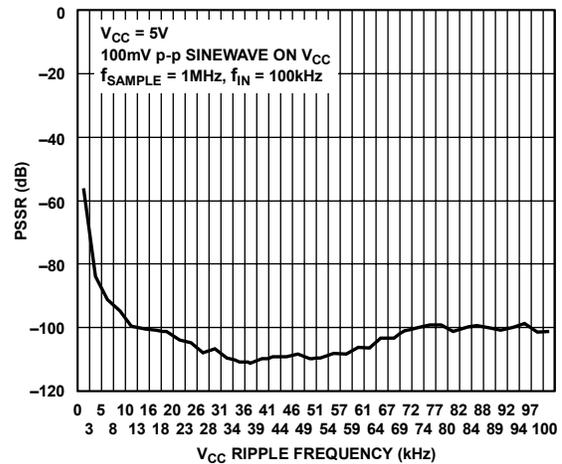
Figure 9. Typical Power Supply Rejection Ratio (PSRR)
