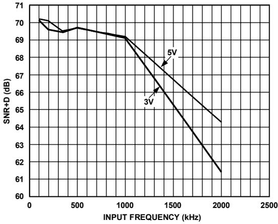
Figure 4. Typical SNR + D vs. Input Tone
