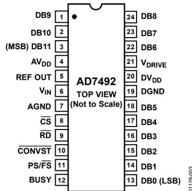
Figure 3. Pin Configuration
