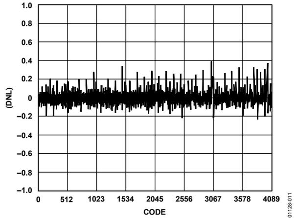
Figure 11. Typical DNL for 2.75 V @ 25°C
