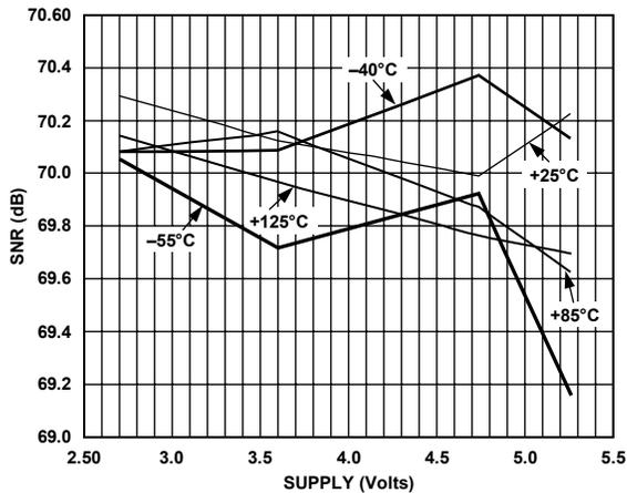
Figure 6. Typical SNR vs. Supply
