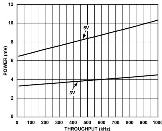
Figure 25. Power vs. Throughput (Mode 1 @ 5 V and 3 V)
