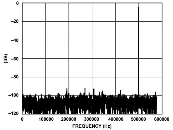
Figure 7. Typical SNR @ 500 kHz Input Tone
