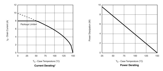
\* The power dissipation  $P_D$  is based on  $T_{J(max)} = 175$  °C, using junction-to-case thermal resistance, and is more useful in settling the upper dissipation limit for cases where additional heatsinking is used. It is used to determine the current rating, when this rating falls below the package limit.
