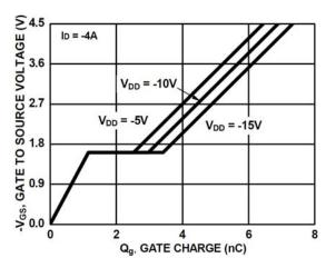
Figure 14. Gate Charge vs Gate to Source Voltage
