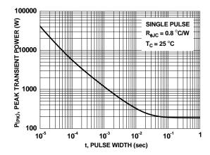
Figure 12. Single Pulse Maximum Power Dissipation
