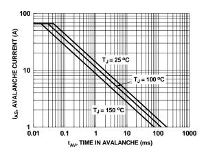
Figure 9. Unclamped Inductive Switching Capability
