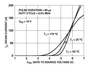
Figure 5. Transfer Characteristics
