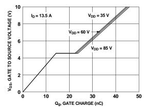
Figure 7. Gate Charge Characteristics
