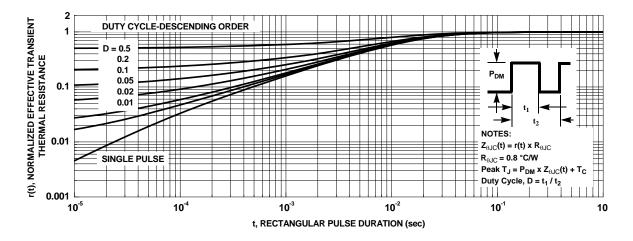
Figure 13. Junction-to-Ambient Transient Thermal Response Curve
