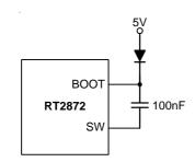
Figure 2. External Bootstrap Diode
