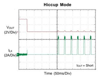
Figure 5. Hiccup Mode Under-Voltage Protection
