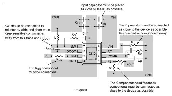
Figure 8. PCB Layout Guide
