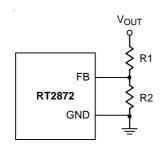
Figure 1. Output Voltage Setting
