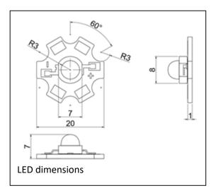
If mounting the LED with metal fixings take care to ensure that the PCB pads are not shorted out.
