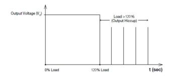
Additionally, if the  $I_O$  is < 120% but > 100% for a prolong period of time (depending on the load), the Over Temperature Protection (OTP) will be activated due to high temperature on critical components. The power supply will then go into "Hiccup mode" until power supply cool down.
