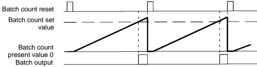
The batch count output holds until reset by the batch count reset. The present value of the batch count advances continuously.
