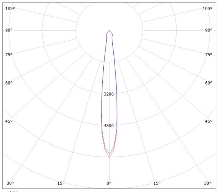
cd/klm \_\_\_\_\_ C0 - C180 \_\_\_\_\_ C90 - C270 NOTE: The typical divergence will be changed by different color, chip size and chip position tolerance. The typical total divergence is the full angle measured where the luminous intensity is half of the peak value.
