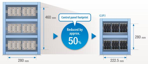
Example: Installation of 18 SSRs constituted for three-phase heaters (6 channels)
