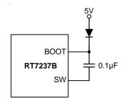
Figure 2. External Bootstrap Diode
