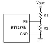
Figure 1. Output Voltage Setting
