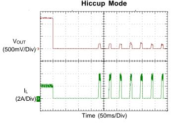
Figure 5. Hiccup Mode Under Voltage Protection
