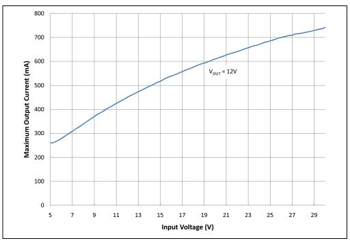
FIGURE 2-1: Typical Maximum Output Current vs. Input Voltage
