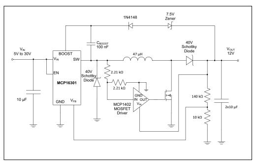
FIGURE 1-1: Typical MCP16301 Buck-Boost Application.
