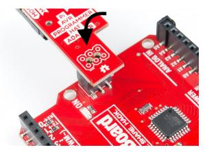
• Plug in a USB cable from the Pi to the RedBoard. This will provide power to the RedBoard. You could also opt to power the board via the barrel jack if you wish.
