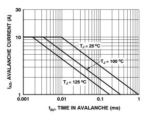
Figure 9. Unclamped Inductive Switching Capability
