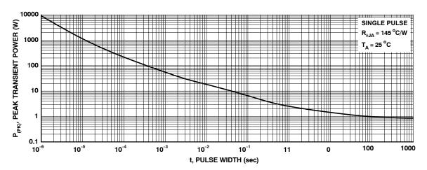
Figure 11. Single Pulse Maximum Power Dissipation
