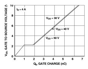
Figure 7. Gate Charge Characteristics
