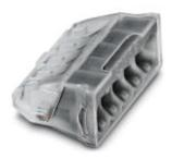
5-pos. socket terminal block with spring-cage connection, for toolless wiring with push-in connection method, for one and multi-strand conductors with a cross section of 0.5 to 2.5 mm², insulation housing transparent.
