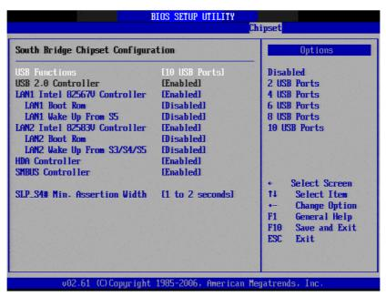
**Figure 3.26 South Bridge Configuration**
