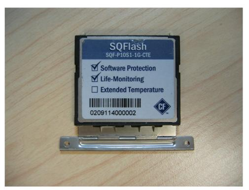
Figure 2.15 Put CF on to the CF tray
