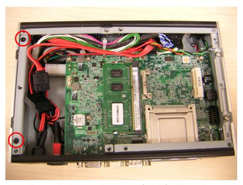
Figure 2.19 Unscrew the screws of the left HDD bracket
