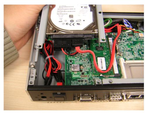
Figure 2.20 Connect the SATA HDD power and signal cables.
