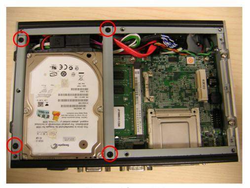
Figure 2.21 Secure HDD
