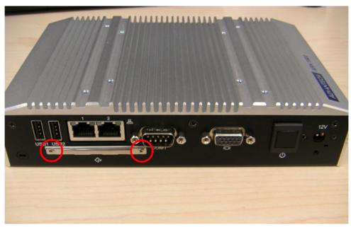
Figure 2.12 Remove the CF door screws
