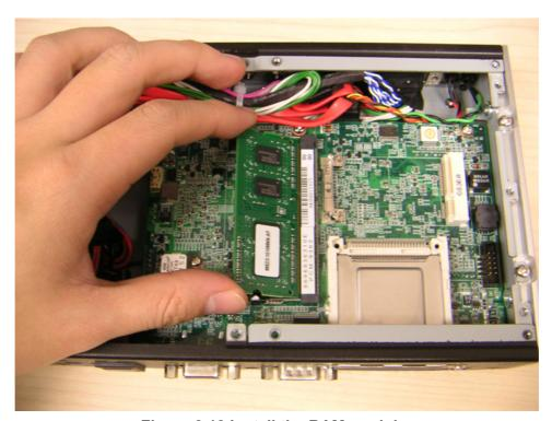
Figure 2.18 Install the RAM module
