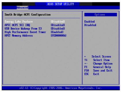
Figure 3.11 Chipset ACPI Configuration
